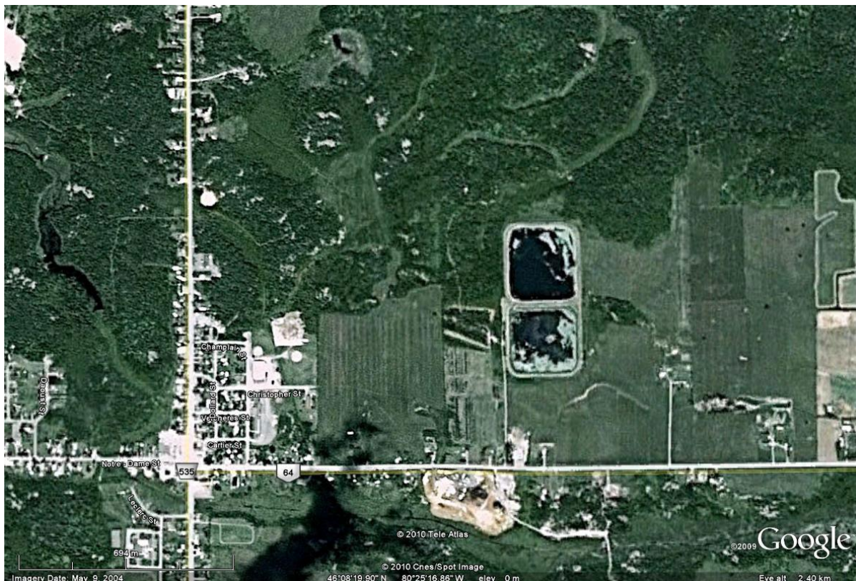
Satellite image of Noelville sewage lagoons off of highway 64. The town of Noelville is to the left of the lagoons.
